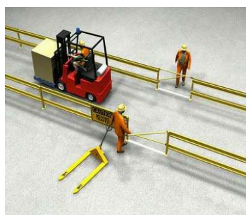
Barriers to separate pedestrians and mobile plant
